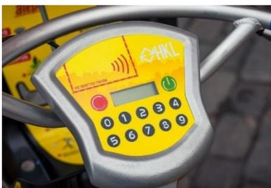
**The "Smooove Box" is the heart of the Smooove solution.** Unlike its main competitors, the communicating technology is embedded directly in the bikes, which are self-powered (thanks to a dynamo), wireless, and are not requiring civil engineering (thanks to solar-powered stations). This revolution simplifies user access, facilitates the deployment of stations, and allows great flexibility in the operation of the projects.
